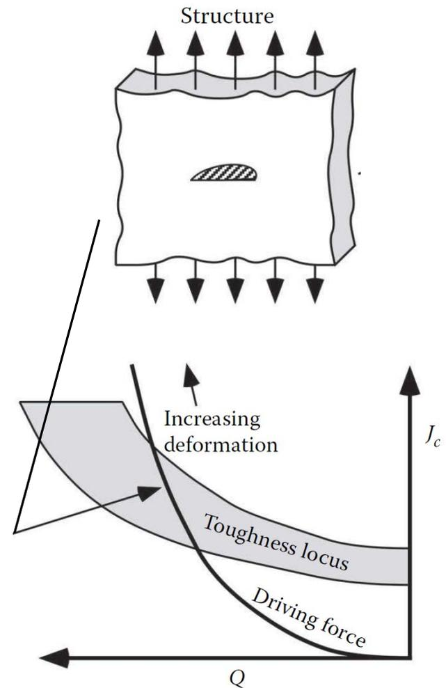
Application of a *J-Q* toughness locus. Failure occurs when the applied *J-Q* curve passes through the toughness locus.
