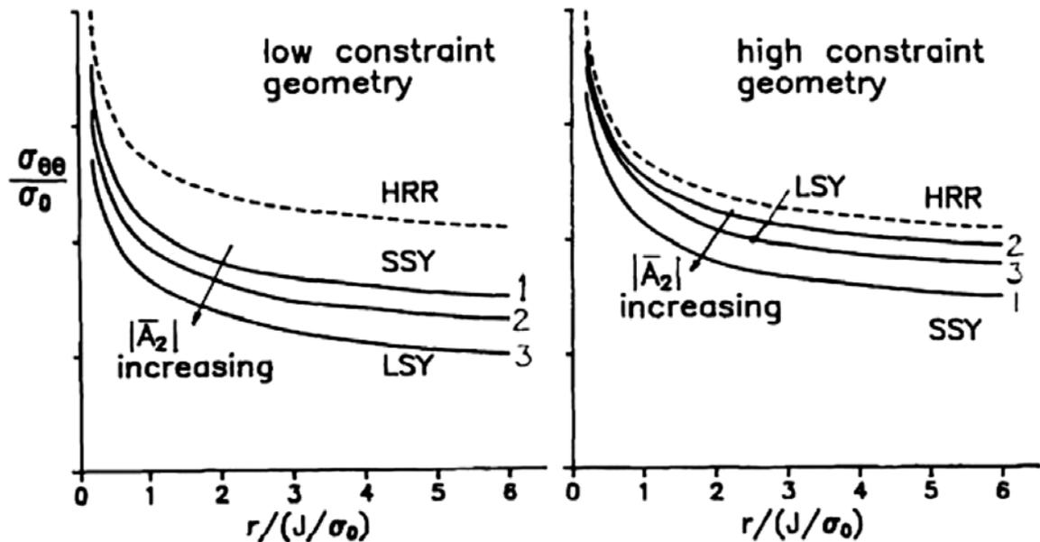
Stress ahead of a crack tip in low and high constraint specimen geometry
