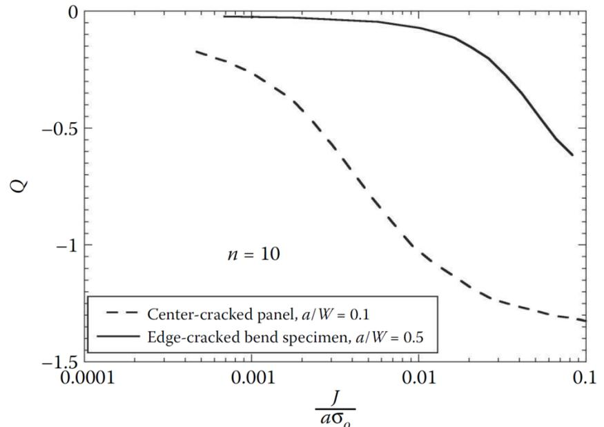
Evolution of the *Q* parameter with deformation in two geometries
