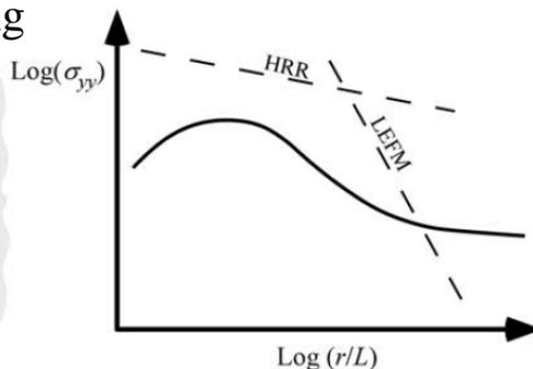
**Large-scale yielding condition:** No single parameter can characterize fracture!
