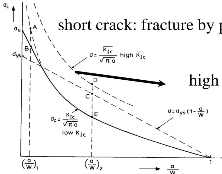
short crack: fracture by plastic collapse!!!
