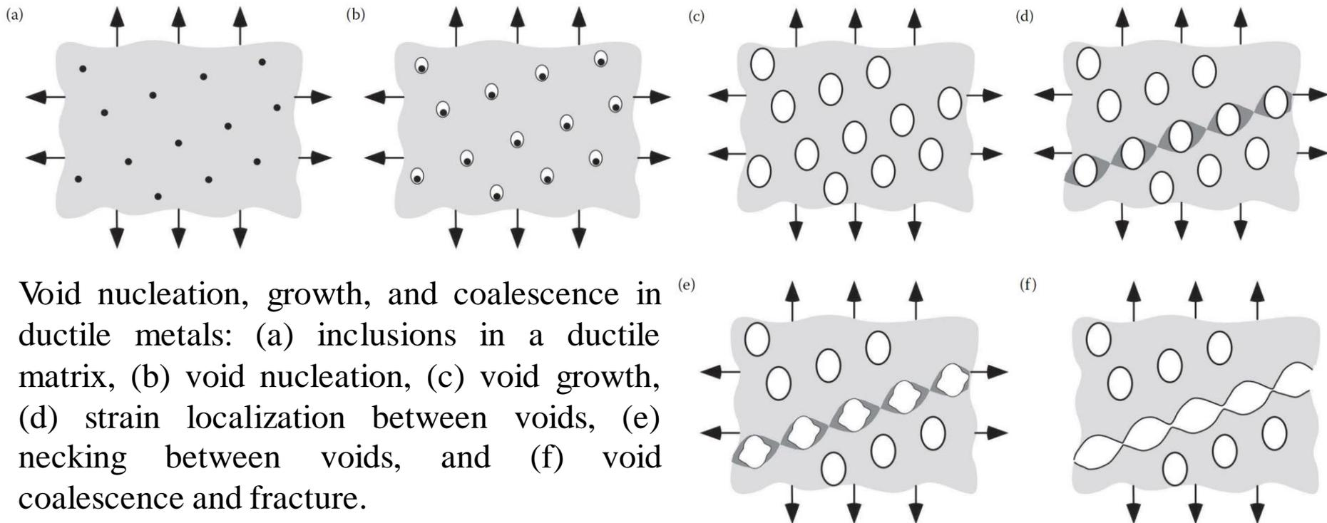
Void nucleation, growth, and coalescence in ductile metals: (a) inclusions in a ductile matrix, (b) void nucleation, (c) void growth, (d) strain localization between voids, (e) necking between voids, and (f) void coalescence and fracture.
