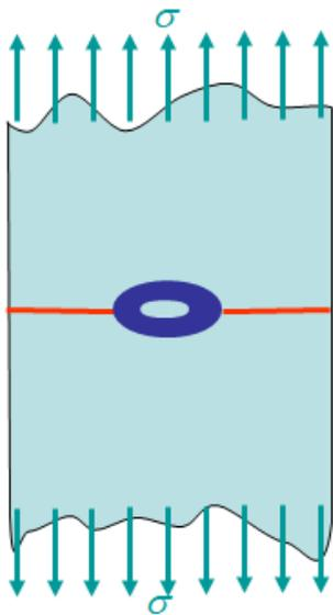
Large yielding: two side cracks subjected to uniform tension.
