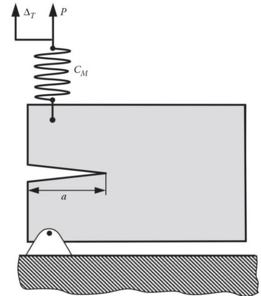
$$\left(\frac{dG}{da}\right)_{\Delta_T} = \left(\frac{\partial G}{\partial a}\right)_P - \left(\frac{\partial G}{\partial P}\right)_a \left(\frac{\partial \Delta}{\partial a}\right)_P \left[ C_M + \left(\frac{\partial \Delta}{\partial P}\right)_a \right]^{-1}$$
