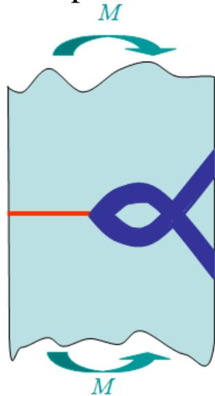
Large yielding: one side crack subjected to a bending moment.
