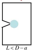
EPFM, J<sub>C</sub> fracture criterion
