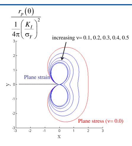
Crack tip plastic zone shapes estimated from the elastic solutions and the von Mises yield criterion: (a) Mode I, (define the approximate boundary between elastic and plastic behavior).
