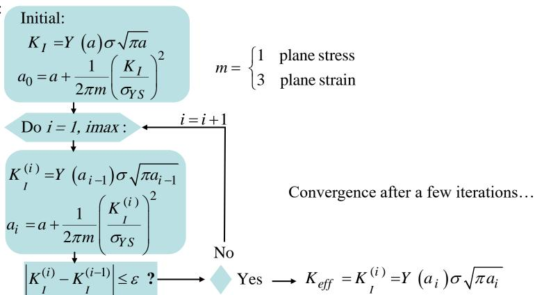
Application: Through-crack in an infinite plate (plane stress):
