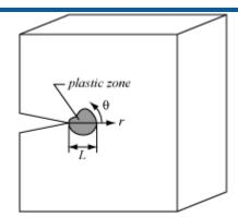
2) Significant difference in the size and shape of mode I plastic zones.
