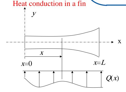
A(x) = cross section at x Q(x) = heat input per unit length perunit time [J/sm]<math>k(x) = thermal conductivity [J/°C ms]T(x) = temperature of the fin at x
