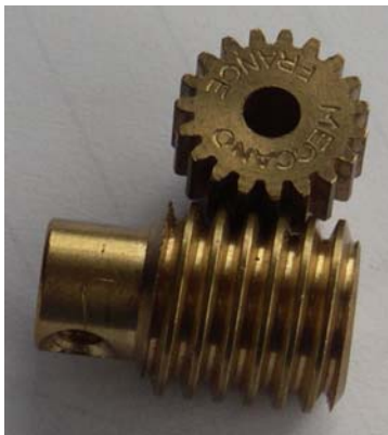
Worm Gear and Pinion
